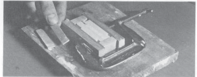
For parts that were to be fully encased such as the stone columns, the upper three quarters were included in the first mold and the bottom surface included in the second. The first mold was notched so that when the second was poured it registered properly and easily. The surface was coated with Vaseline spread thinly. The dam was then raised with spacers to a new height allowing the second coating of rubber to be poured.
