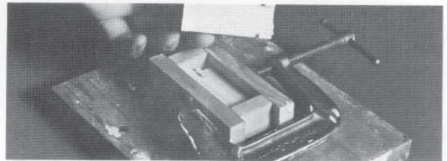
For parts that were to be fully encased such as the stone columns, the upper three quarters were included in the first mold and the bottom surface included in the second. The first mold was notched so that when the second was poured it registered properly and easily. The surface was coated with Vaseline spread thinly. The dam was then raised with spacers to a new height allowing the second coating of rubber to be poured.
