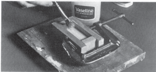
For parts that were to be fully encased such as the stone columns, the upper three quarters were included in the first mold and the bottom surface included in the second. The first mold was notched so that when the second was poured it registered properly and easily. The surface was coated with Vaseline spread thinly. The dam was then raised with spacers to a new height allowing the second coating of rubber to be poured.
